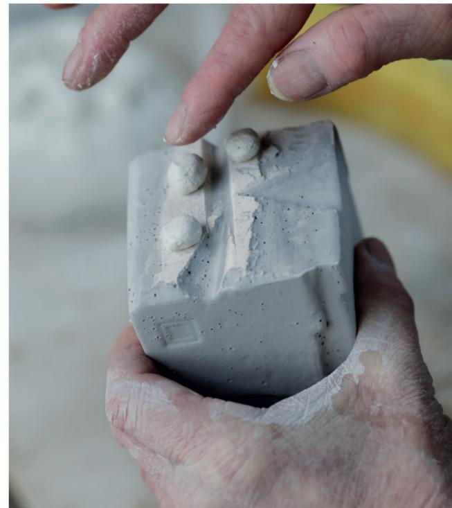
**25** As my glazes are applied thickly and I fire to a very high temperature (cone 10 – around 1310°C), my glazes often run. To prevent the work gluing itself to the kiln batt, I give all my shelves a thick coat of batt wash and wad every piece prior to placing it in the kiln. My wadding mix is 1/1/1 ratio of alumina hydrate, kaolin and plain flour.
