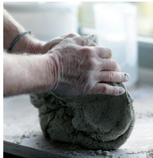
**3** After creating a sandwich of clay and granular material, I spiral wedge it to fully integrate the aggregate into the body. If I am mixing two clays together, I again sandwich alternating layers of clay then spiral wedge until they are fully blended.
