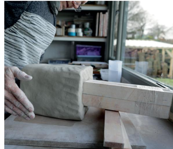
**9** When the wooden insert has been pushed to the desired depth, I flip the piece on its side and start bating the clay back into a controlled shape. I gradually work the displaced clay up and along the wooden insert to increase the height, continually rotating the clay blank to get an even distribution. I also lay some strips of wood under the insert to help control the thickness of the walls. The whole thing is then set aside to slowly dry.
