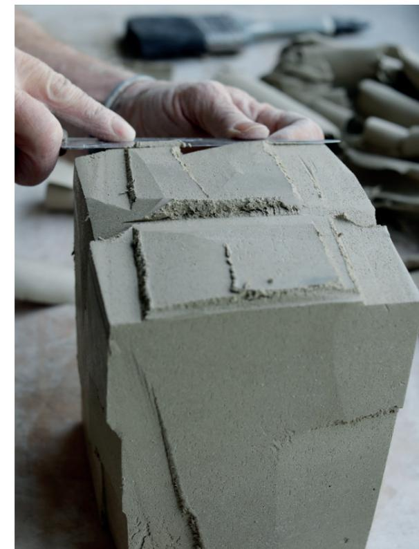
**18** Once the sides of the piece have been carved, I work on the base. I like to create shallow angled undercuts that help to create the illusion of the piece almost floating. The carving and slicing process I have developed may possibly be classed as *Kurinuki* – the Japanese term for a hand-forming process that involves carving a shaped solid block of clay. *Kurinuki* is, however, usually associated with making Yunomi (tea bowls).
