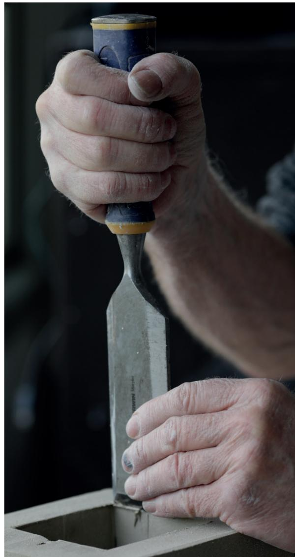
**13** Using a sharp woodworking chisel and the scalpel line as a cutting guide, I pare back each of the interior walls, carefully working my way around each side to produce an interior with crisp sides and edges.
