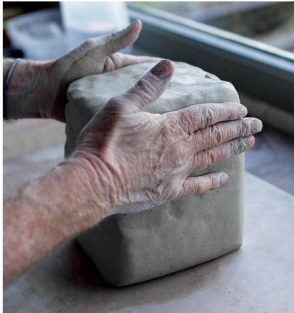
**5** Having prepared my clay body, I decide on the size and proportions of the piece I wish to make. I keep a sketchbook of ideas and will usually make a series of quick drawings prior to starting the making process. The solid lump of plastic clay is knocked and batted into the desired shape or 'blank'.
